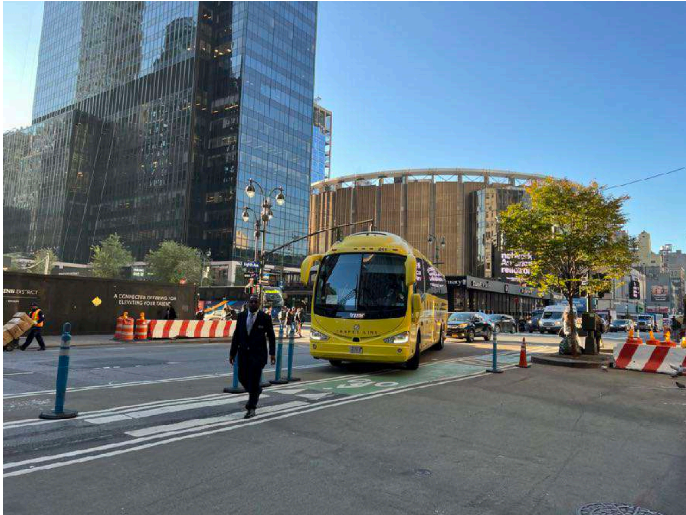
The New Yorker Hotel is inviting busses to cross the bike lane and park on the new sidewalk. More permanent vertical delineators are needed here and some hard separation between the small outer pedestrian island and the parking area.
