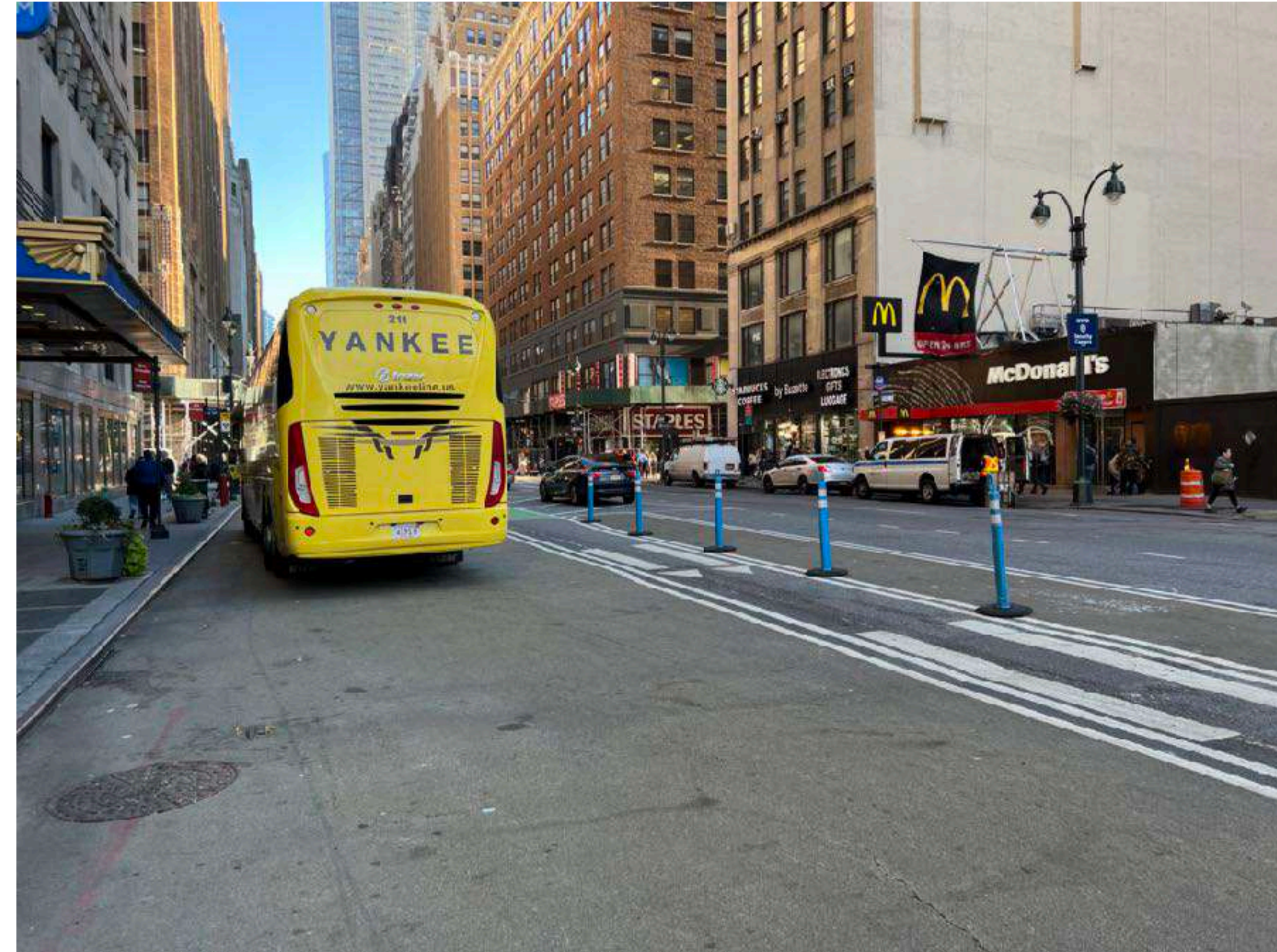
The New Yorker Hotel is inviting busses to cross the bike lane and park on the new sidewalk. More permanent vertical delineators are needed here and some hard separation between the small outer pedestrian island and the parking area.
