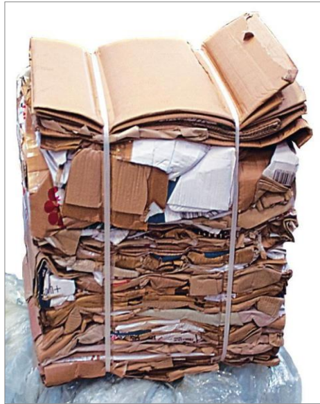
Cardboard baling reduces volume by 30%
