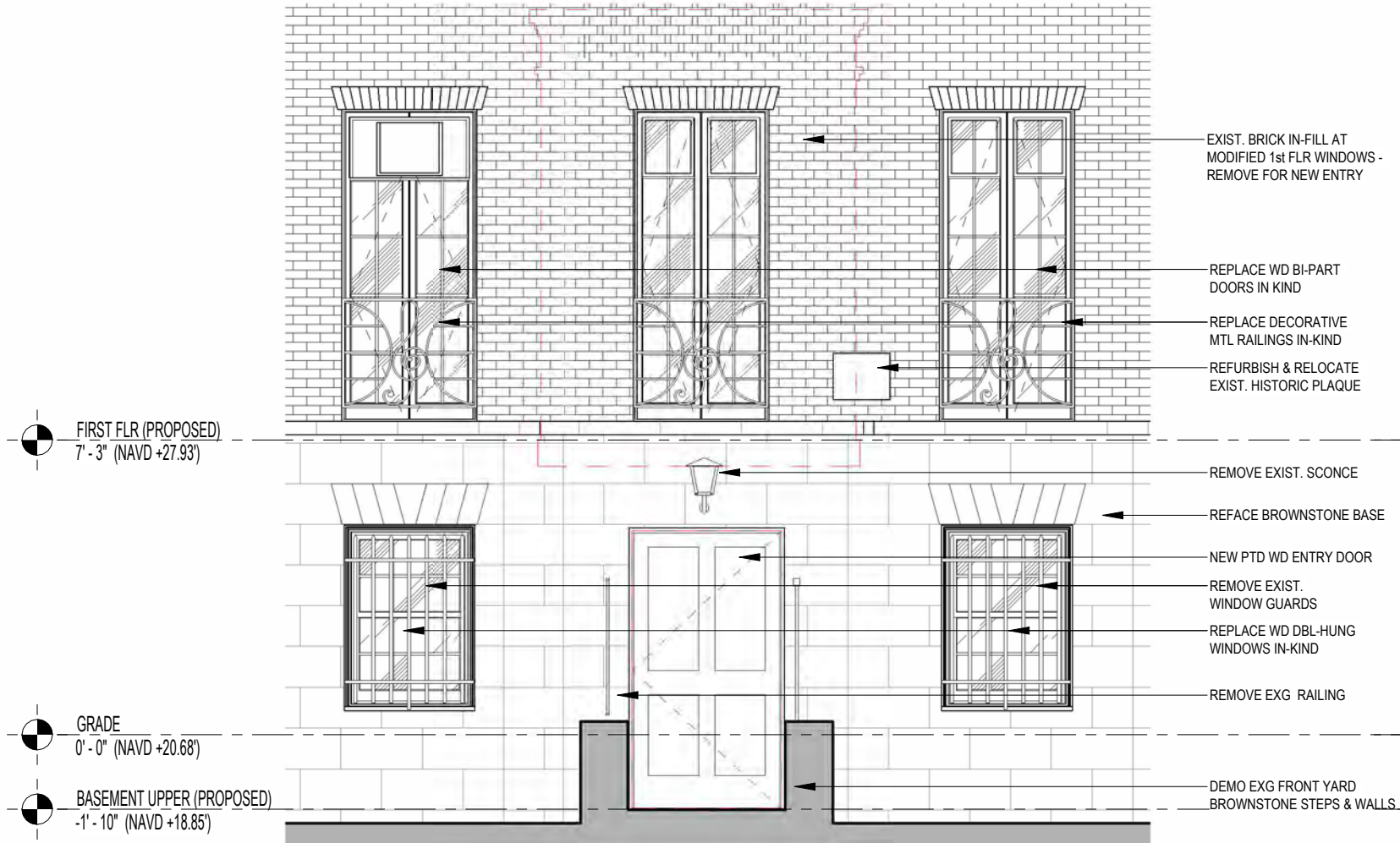
ENLARGED ELEVATION - EXISTING ENTRY SCALE: 1/4" = 1'-0"
