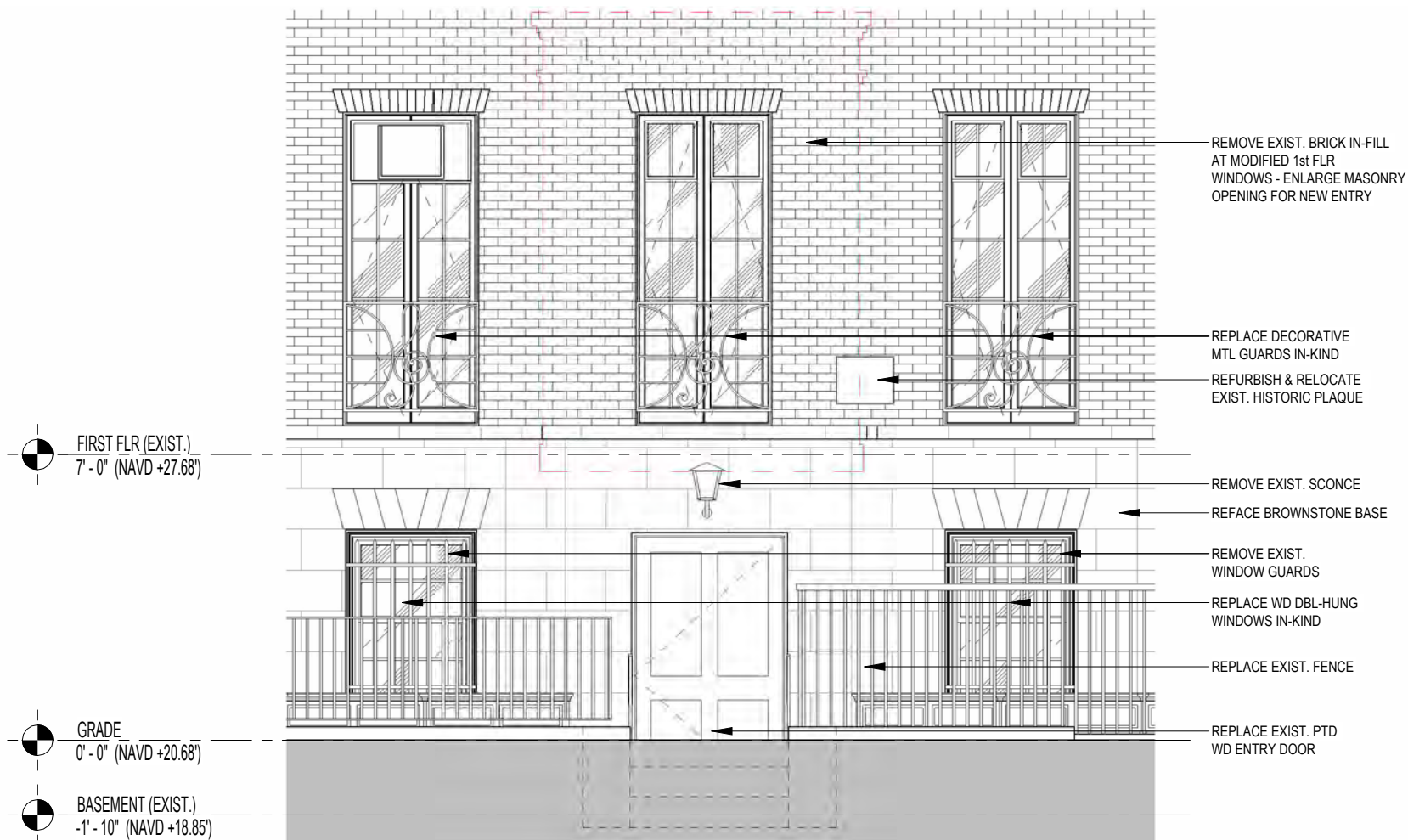
ENLARGED ELEVATION - EXISTING ENTRY SCALE: 1/4" = 1'-0"
