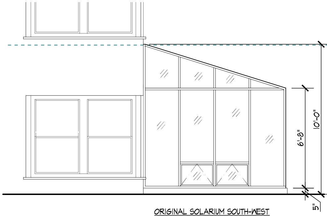
Original Solarium South Elevation Scale: 1/4"= 1'-0"
