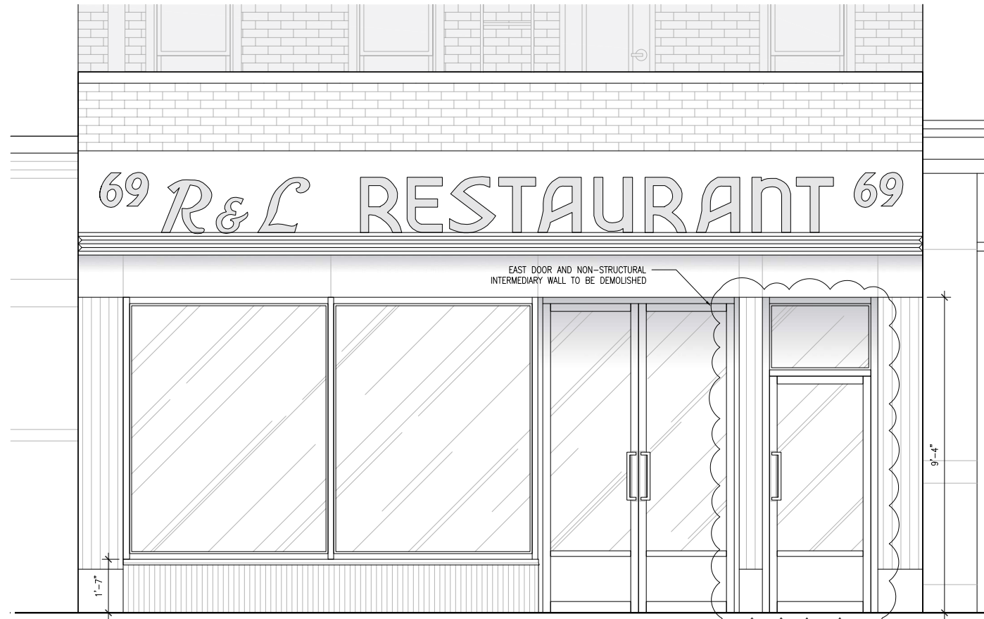
EXISTING FIRST FLOOR SOUTH ELEVATION
