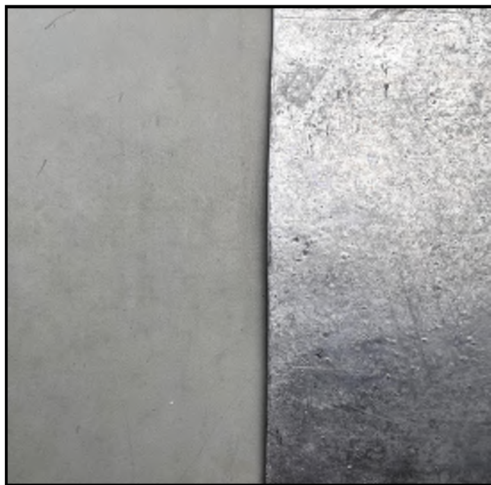
ROOFTOP BULKHEAD, GUTTERS & CLERESTORY WINDOW CLADDING: TIN-ZINC COATED COPPER (L: WEATHERED/R: NEW)
