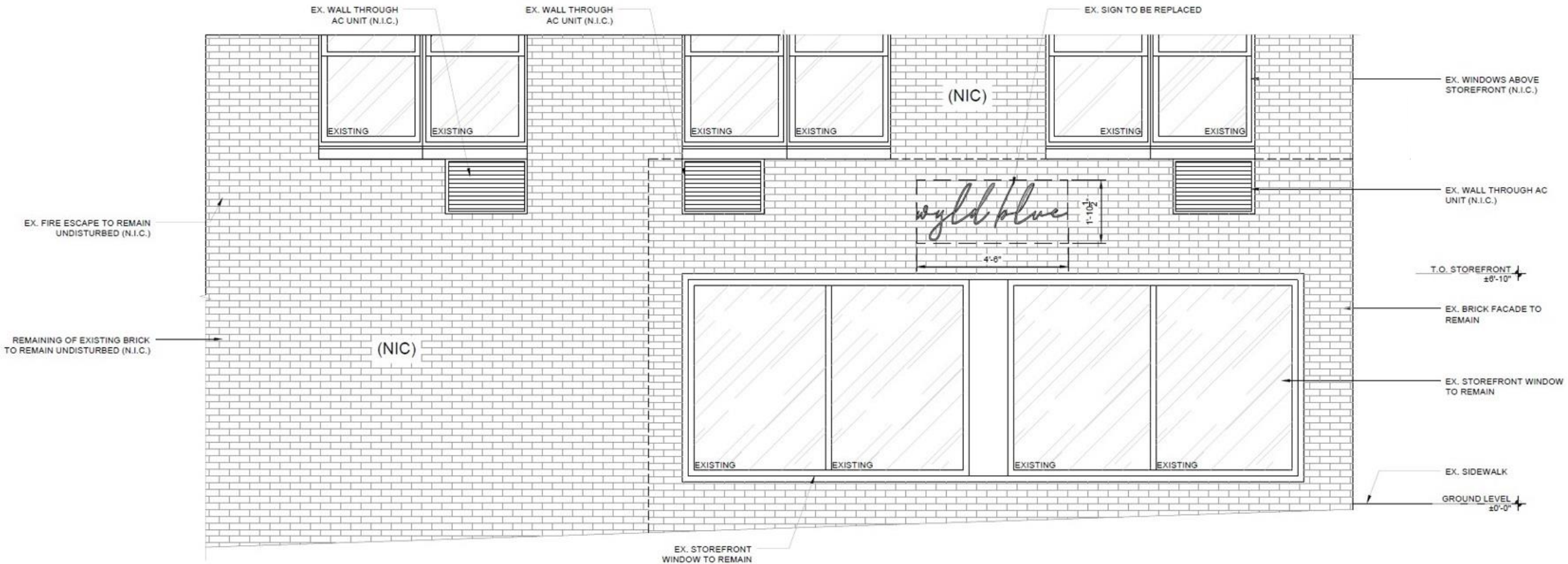
3 W 10TH STREET EXTERIOR EXISTING ELEVATION SCALE: 1/2" = 1'-0"
