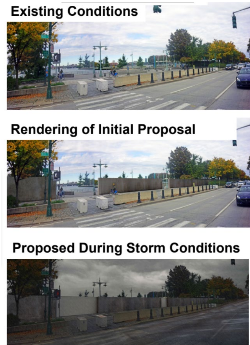
Fig. 6: Rough Rendition of Floodwall along West Street
