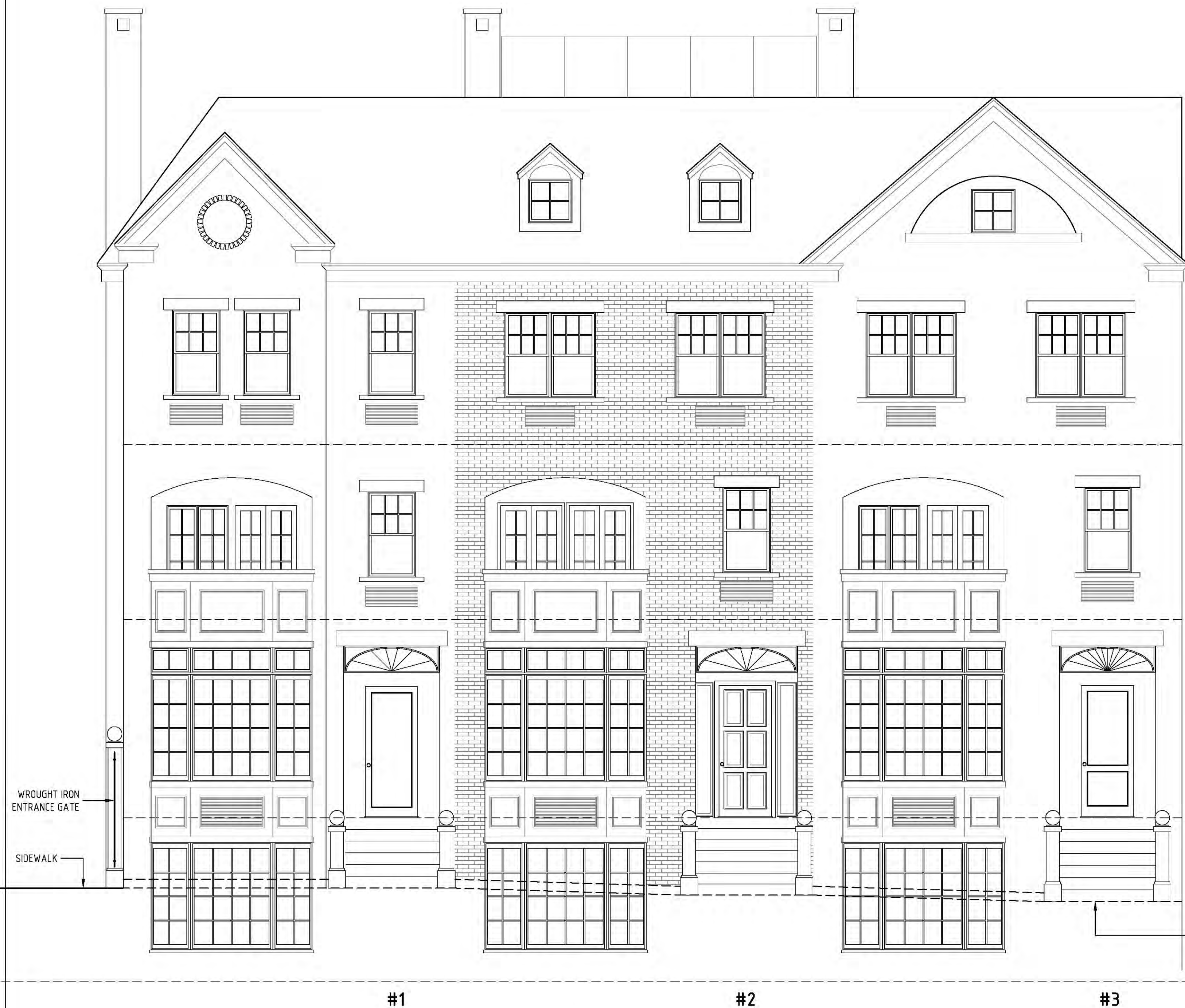
1 EXTERIOR ELEVATION MEWS LOOKING NORTH Scale: 1/4" = 1'-0"
