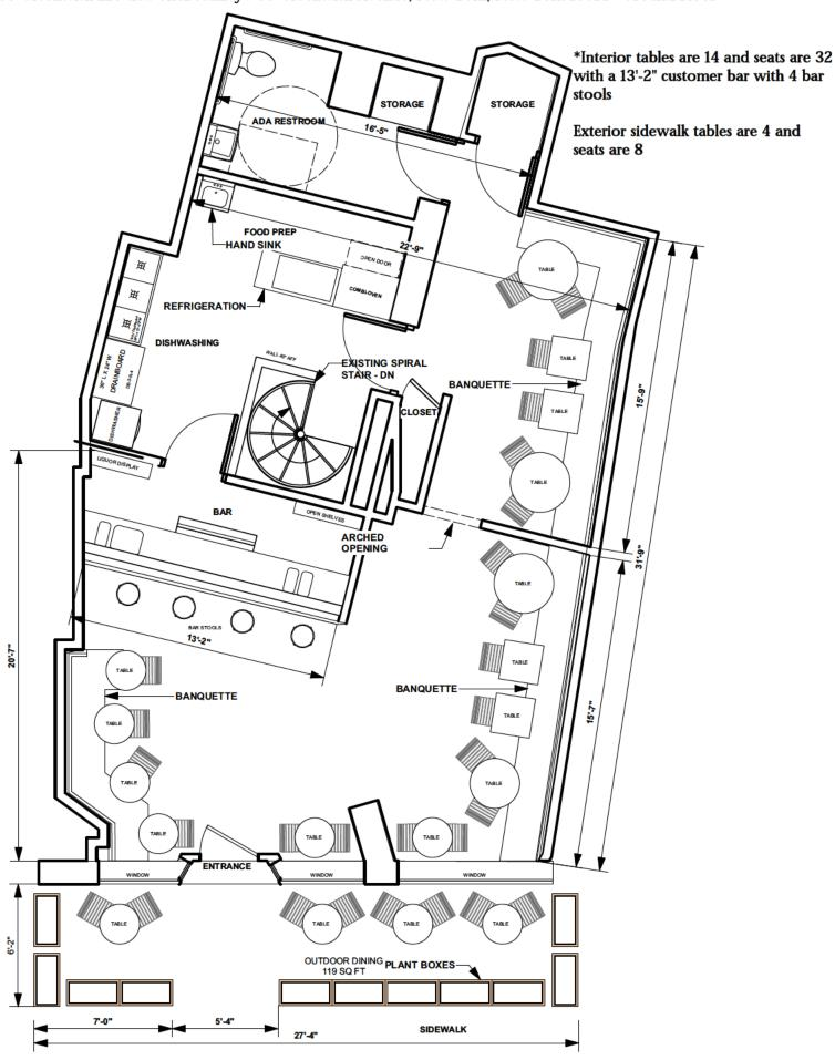
GROUND FLOOR PLAN - +/-921 GSF - Scale: 3/16" = 1'-0"
