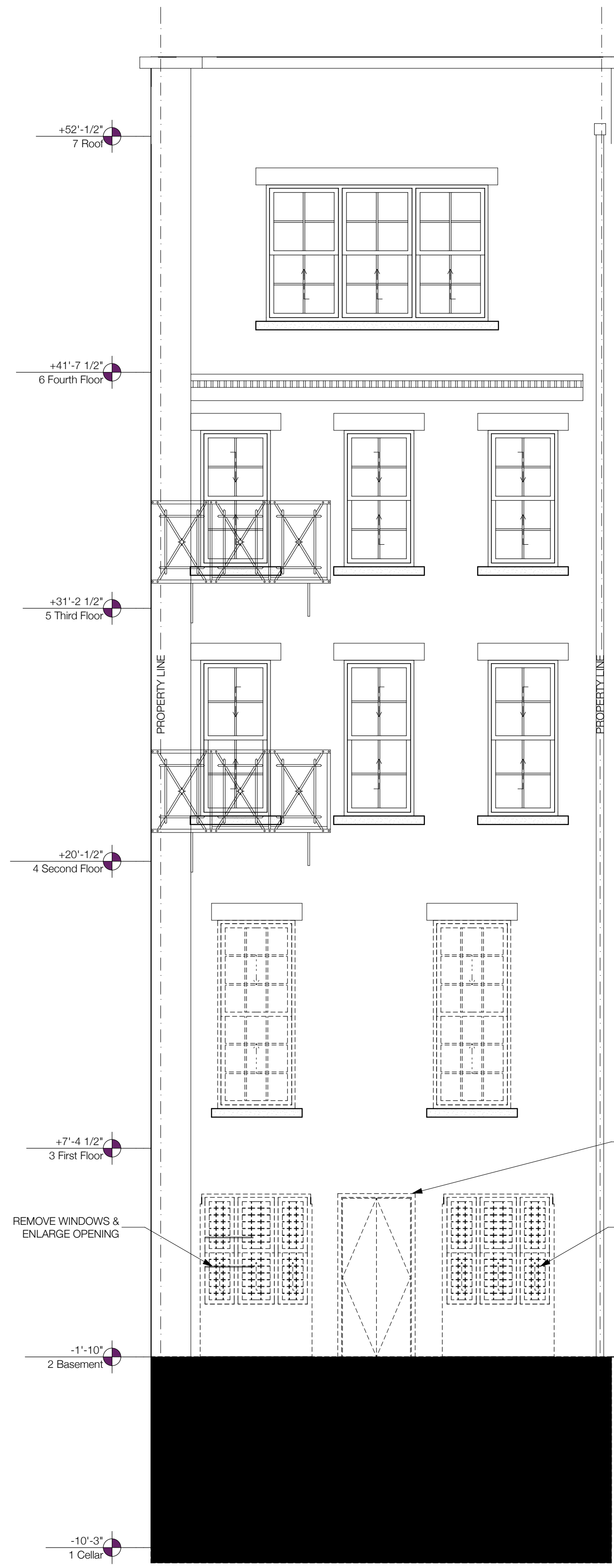
3 Demolition Rear Elevation SCALE: 1/4" = 1'-0"
