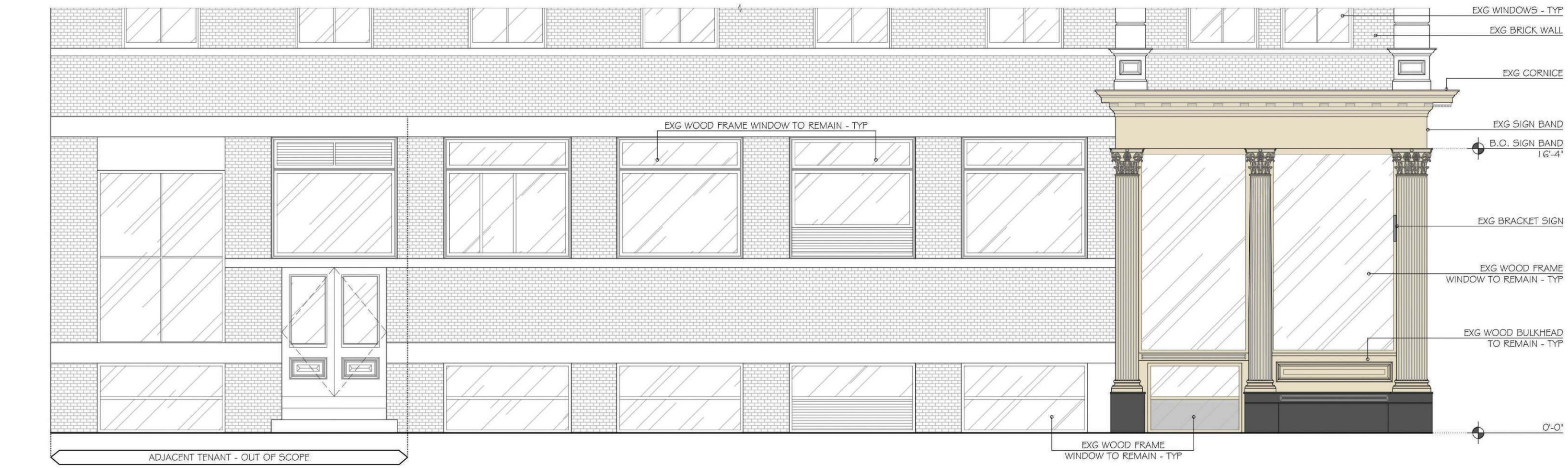
1 EXG STOREFRONT ELEVATION (GREENE ST) Scale: 1/4"=1'-0"
