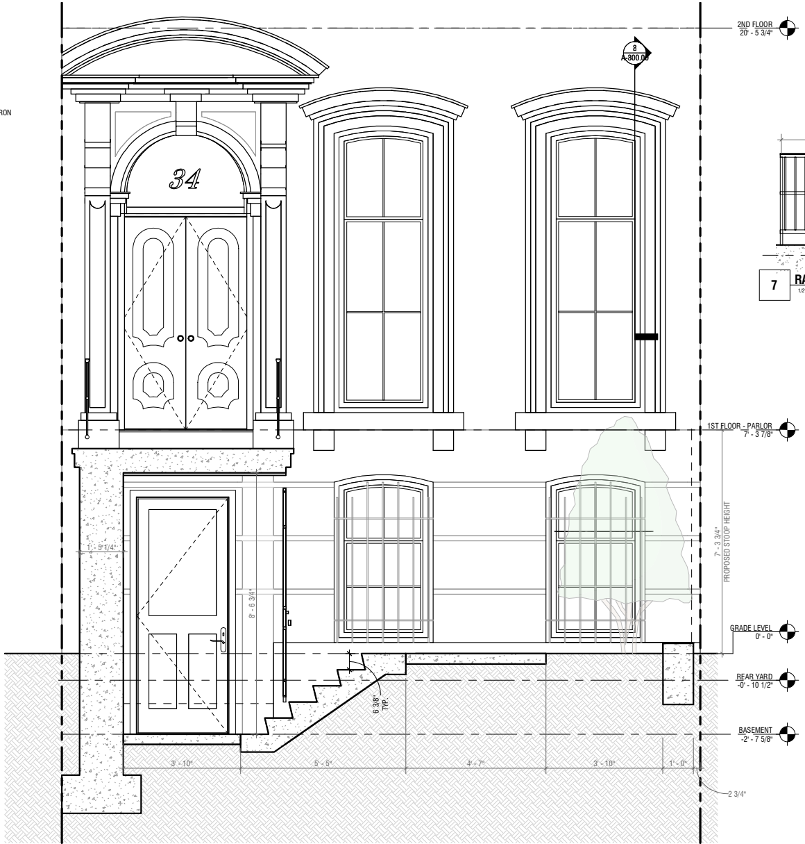
8 EXTERIOR SECTION @ BASEMENT ENTRANCE 1/2" = 1/8"
