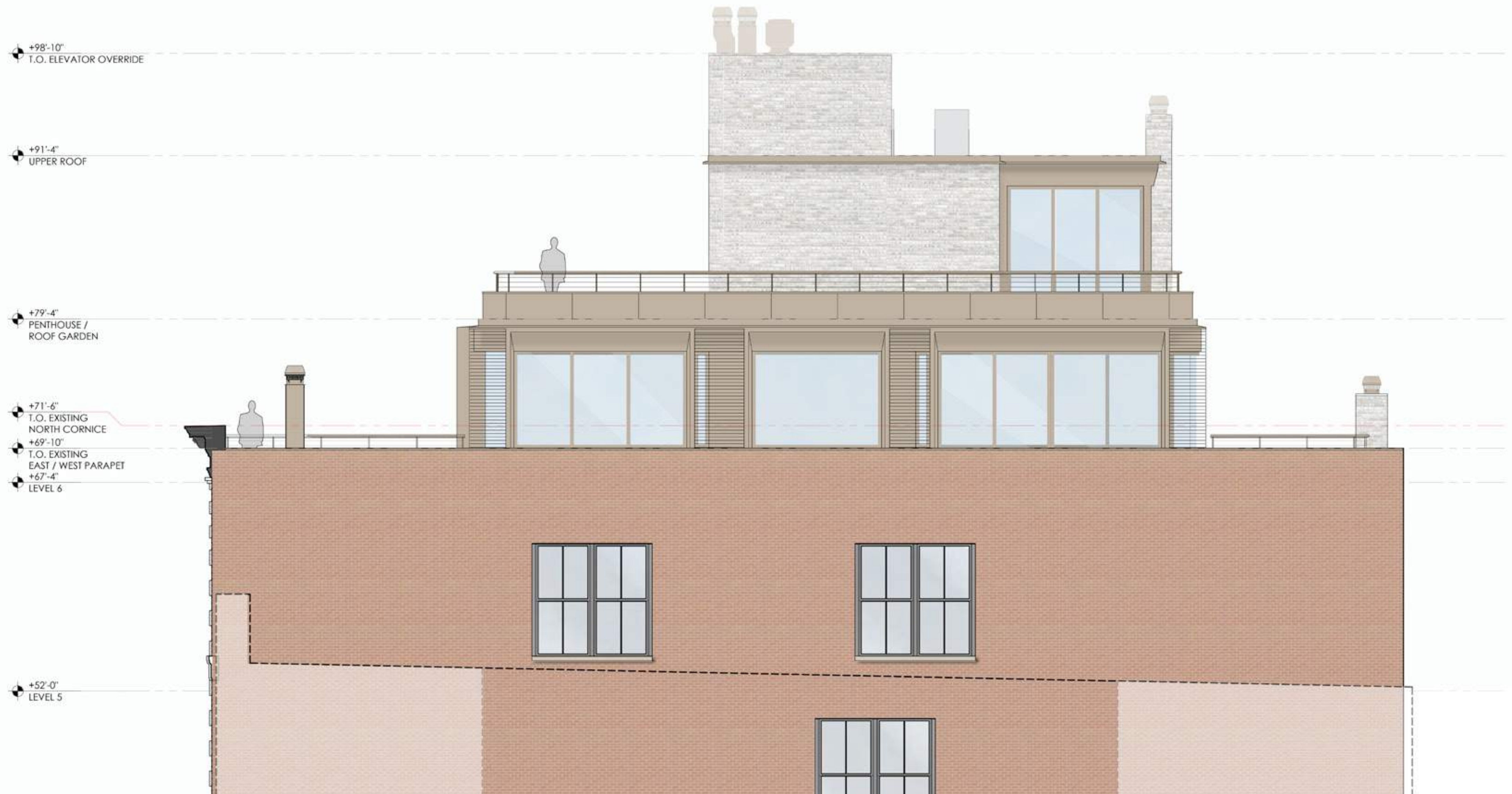
Proposed 6th Floor & Mezzanine enlarged west elevation
