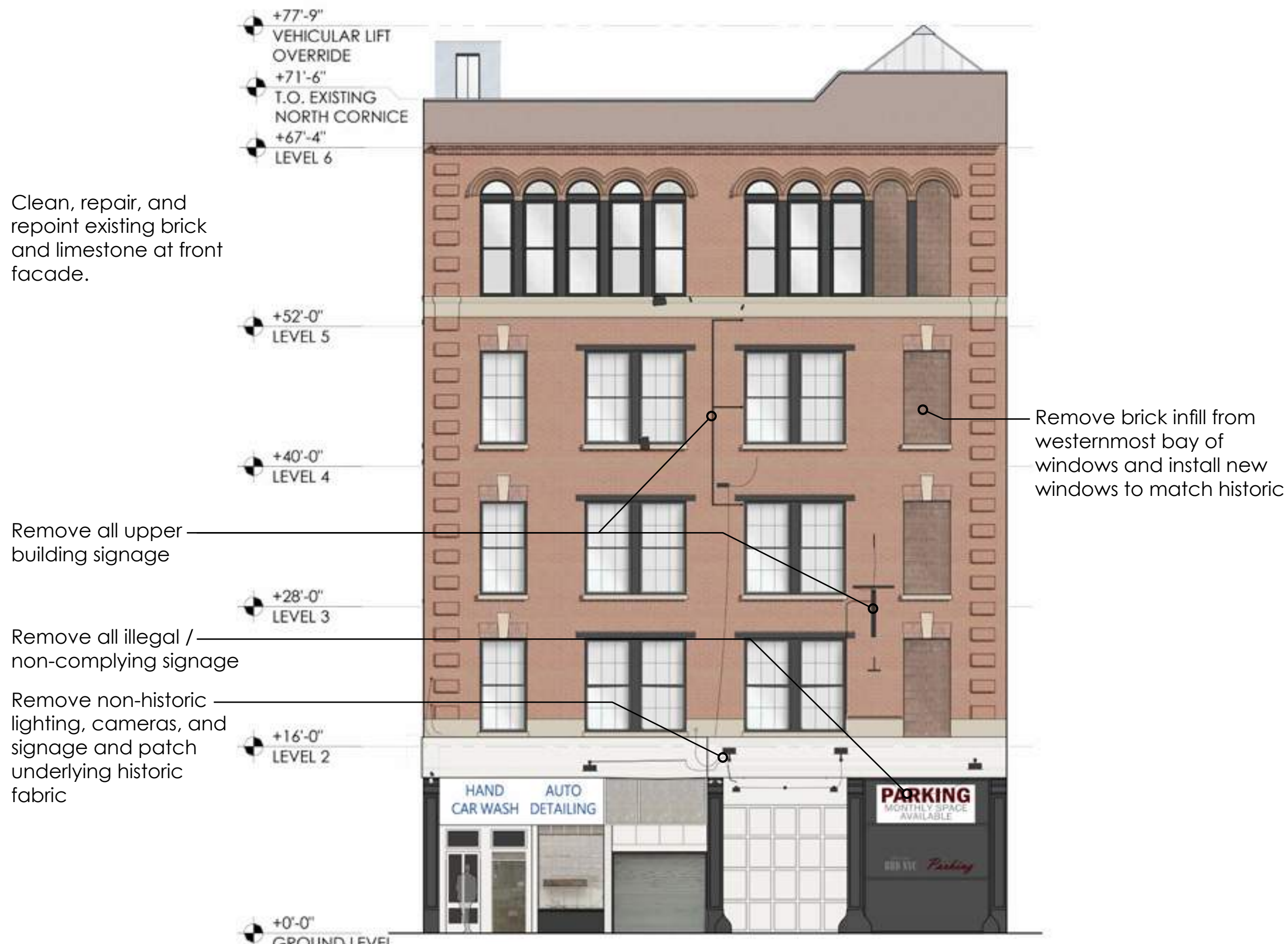
Existing North Elevation
