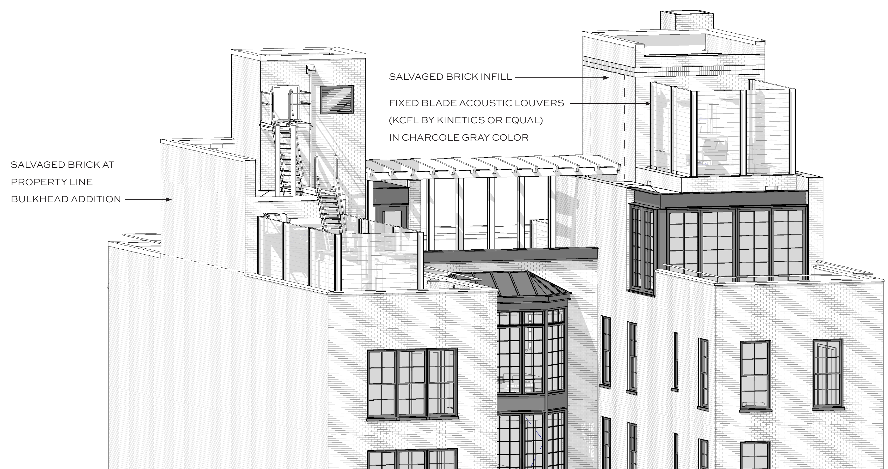
ROOF AND BULKHEADS REAR VIEW - PROPOSED
