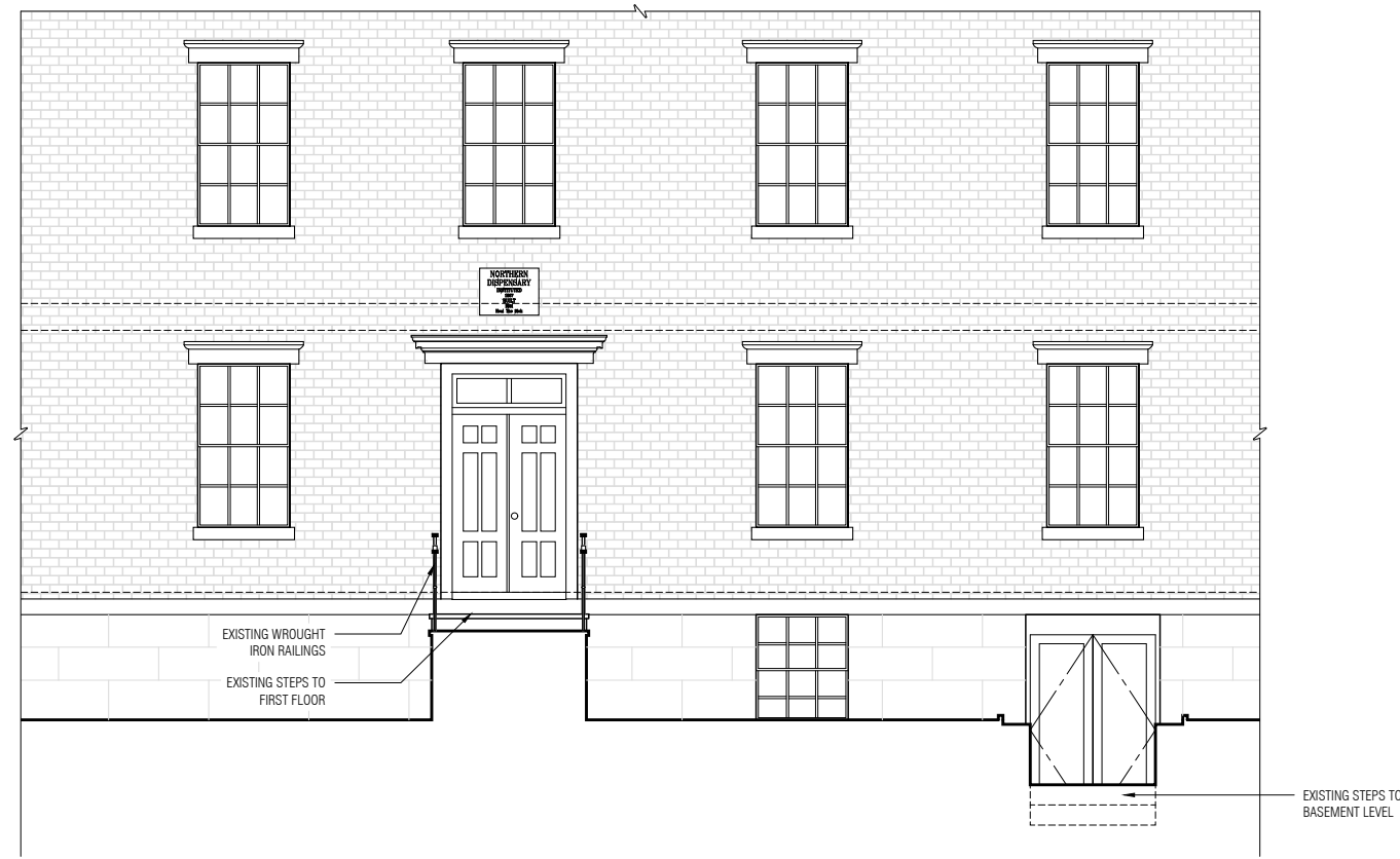
1 ENLARGED EXISTING WEST ELEVATION SECTION IN AREA OF PROPOSED ALTERATION EX-202 SCALE: 1/4" = 1'-0"
