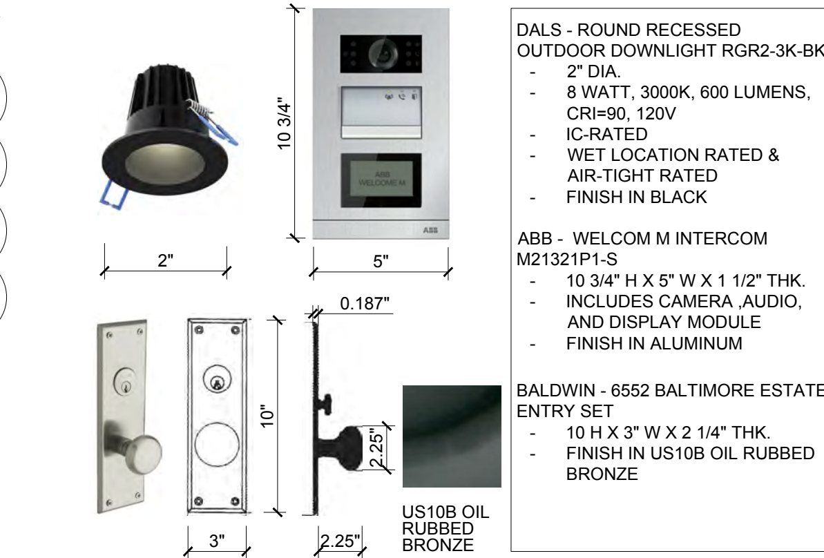
03 PROPOSED DOOR HARDWARE, RECESSED LIGHT, & INTERCOM NOT TO SCALE
