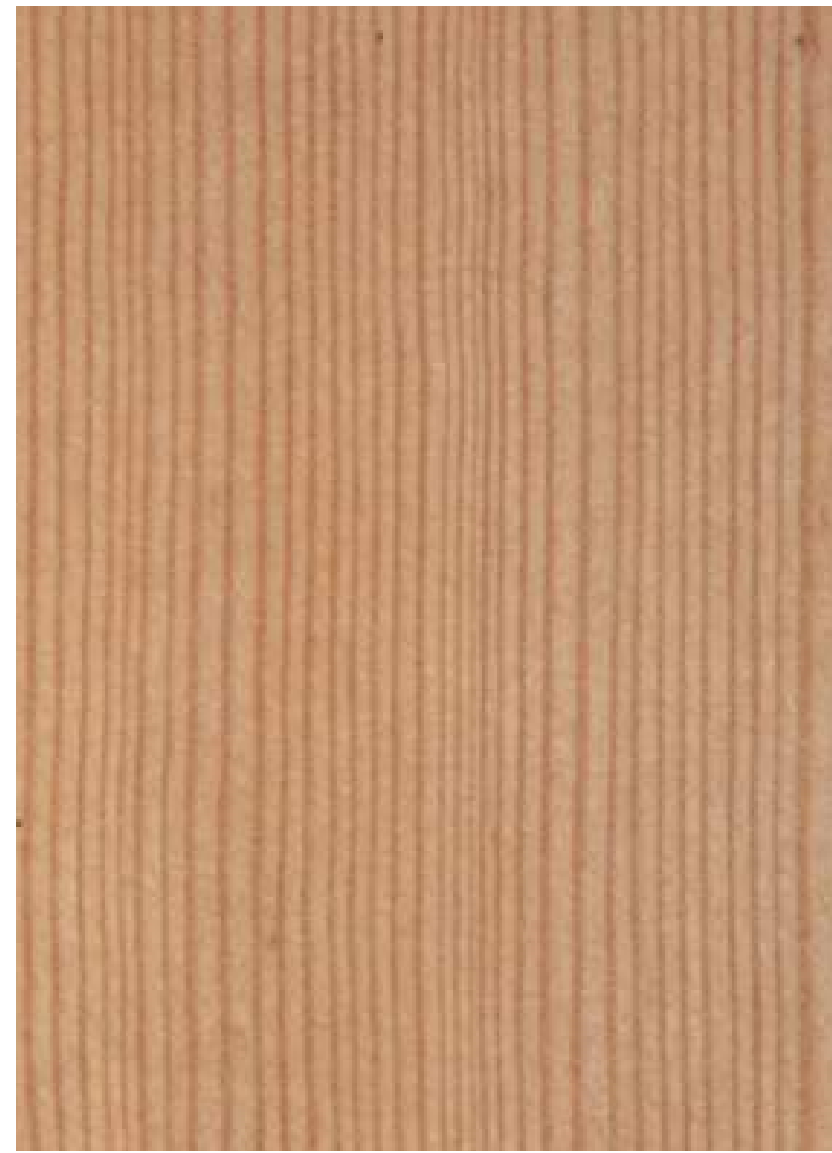
DOUGLASS FIR WOOD FRAMING
