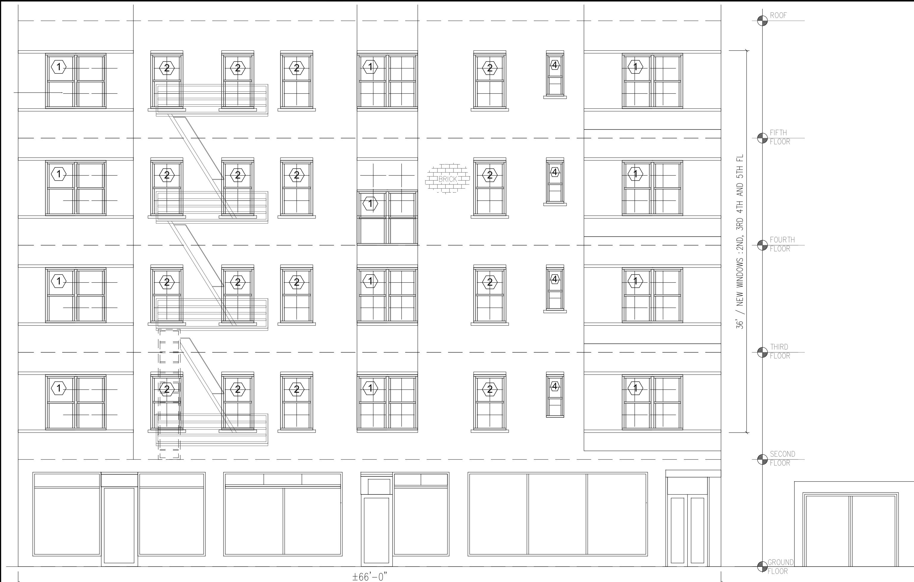
EXTG WEST / HUDSON STREET ELEVATION SCALE: 3/16"=1'-0"
